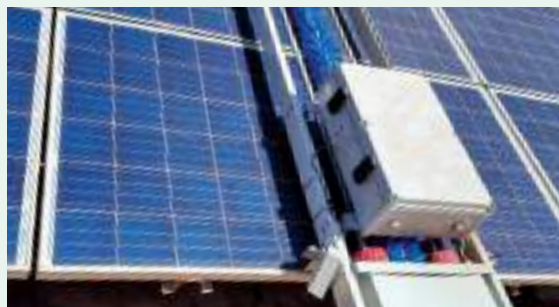
Cleaning of Solar Panels using Robots at Charanka Solar Plant
